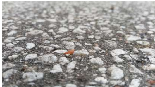
Asphalt incorporating volcanic tuff aggregates
